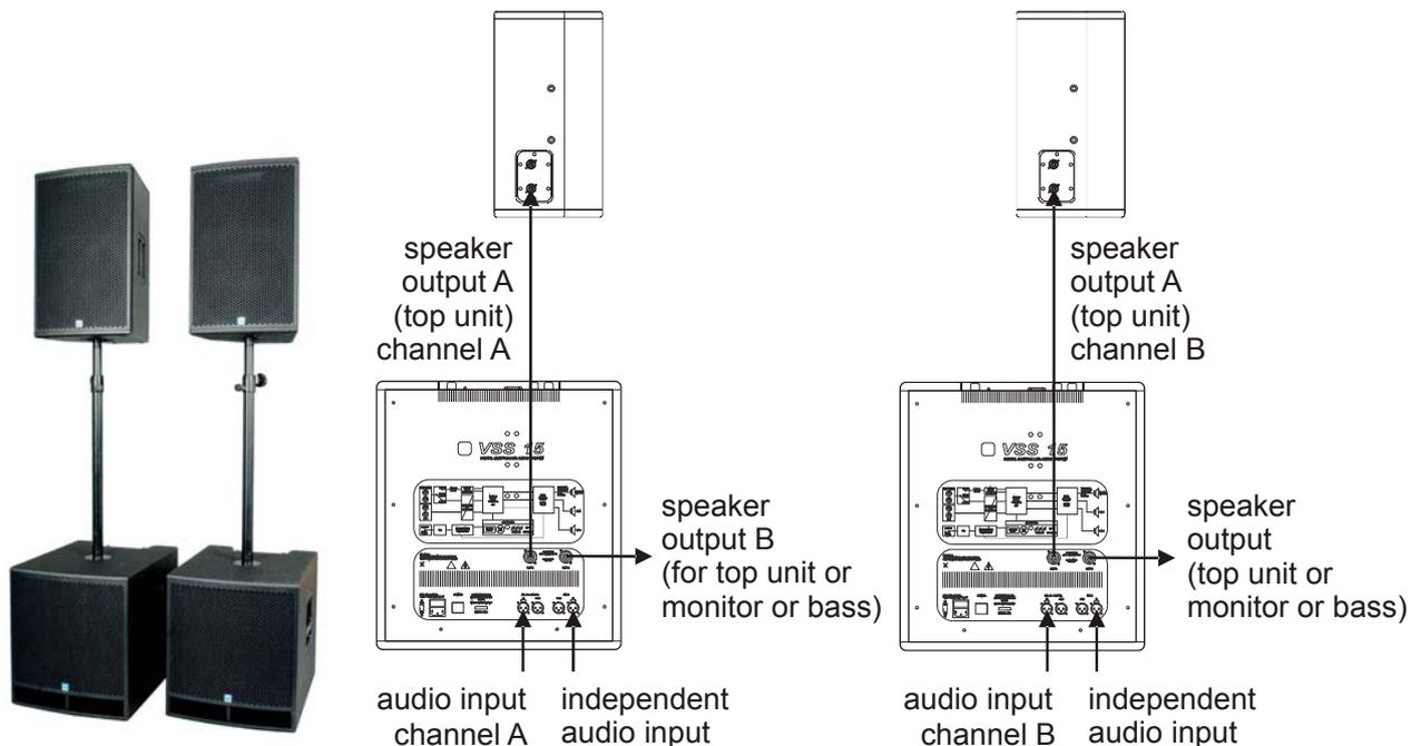
*scheme of the power-output connection of SD 4: from speaker outputs “Out A” into each top unit, speaker outputs “Out B” can be free configurable as monitoring resp. delay-line or as bass extension (depending on preset)*
