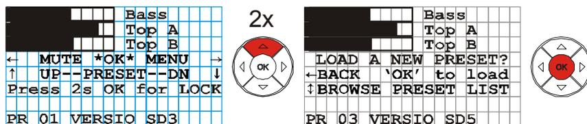
After power on the VSS 15 for the very first time the left graphic appears on the LCD display. You have to press the marked arrow key of the navigation pad two times to select preset 3 „VERSIO SD5“ and confirm with the OK-key. In this case this procedure has to be done once again on the second VSS 15 of the SD5.
