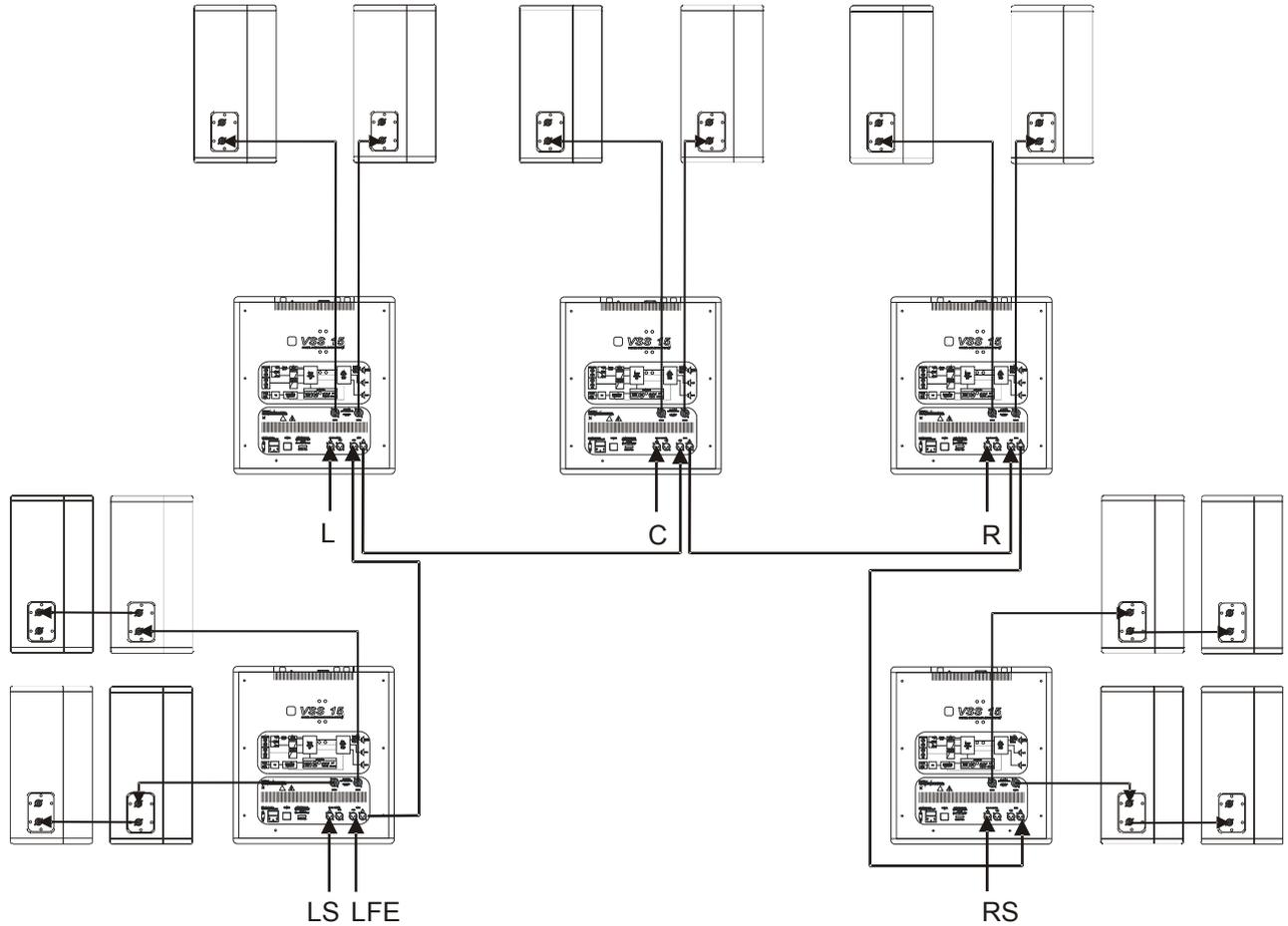
5 x VSS 15 + max. 14x top units (audio inputs & speaker outputs are free configurable).
