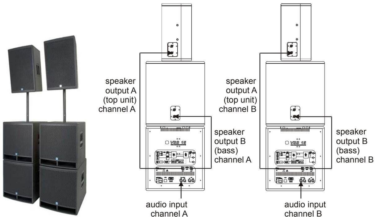
*scheme of the power-output connection of SD 5: from speaker outputs “Out A” into each top unit, from speaker outputs “Out B” into each bass*
