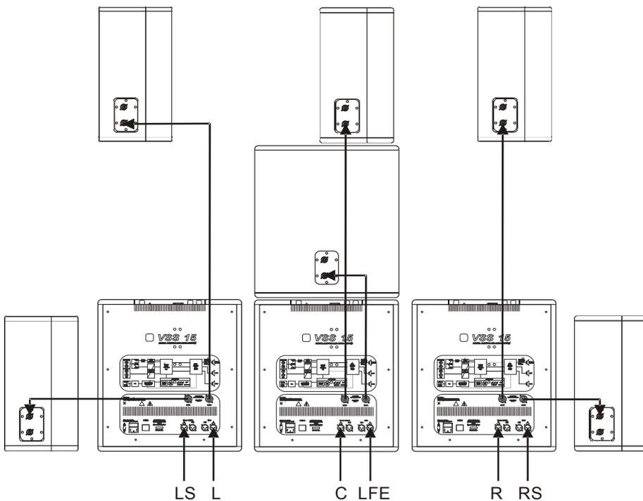
3x VSS 15 + 1x VB 15 + 5x top units (audio inputs & speaker outputs are free configurable).
