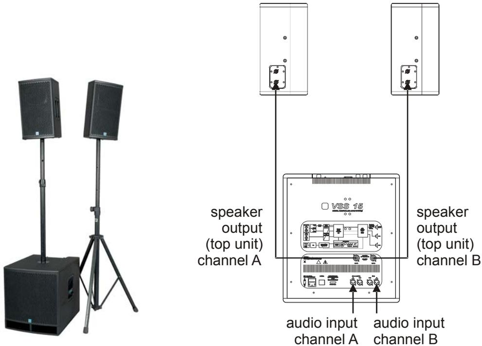
*scheme of the power-output connection of SD 3: from speaker outputs “Out A and Out B” into the top units*
