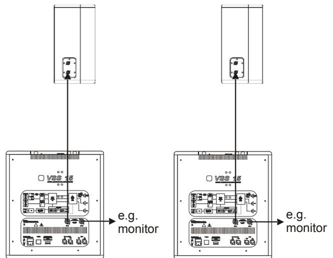
2x VSS 15 + 2x VL 12 + two independently adjustable analogue XLR-inputs (full-range) as well as two speaker outputs (Speakon NL 4): analogue or digital audio signal respectively to input A, input B can respectively be used as an auxiliary
